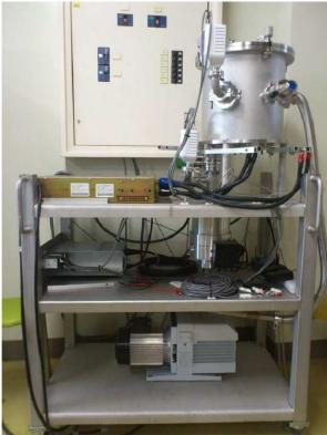
A photograph of a vacuum deposition apparatus. It consists of a stainless steel vacuum chamber mounted on a metal frame. On top of the frame is a control panel with various buttons and a small display screen. A large motor is visible at the bottom of the frame. | 仕様<br>真空チャンバー、<br>ライボルト社ターボ分子ポンプ、<br>250A 直流電源 |
